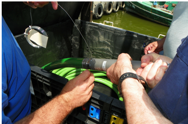
Locking A/D can termination to GeoEel Solid Section.
