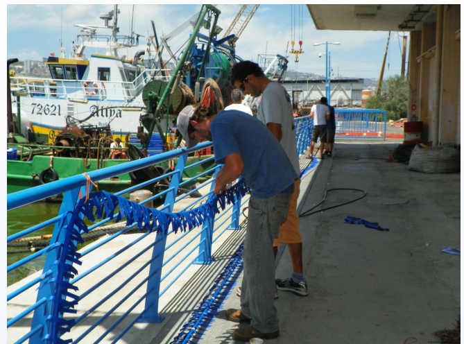
Adding fairing to GeoEel tow cable to reduce noise on the streamer due to cable strumming.
