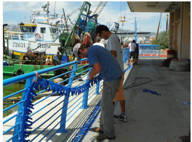
Adding fairing to GeoEel tow cable to reduce noise on the streamer due to cable strumming.
