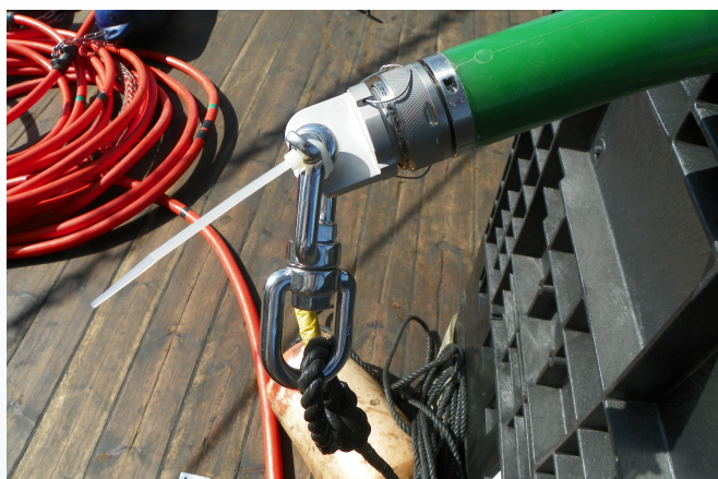
GeoEel Termination with tail buoy
