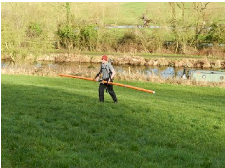
CMD Explorer survey up and down a slope integrating geospatial positions.
